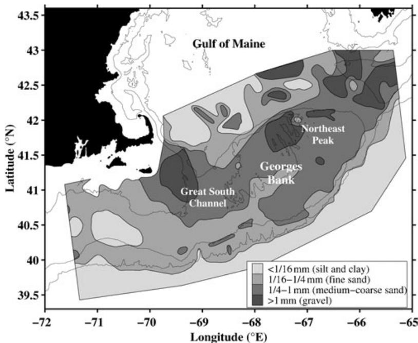
**Figure 3.** Bottom sediment grain size over Georges Bank showing distributions of silt and clay, fine sand, medium-to-coarse sand, and gravel (after Twichell *et al.*, 1987; republished from Schlee, 1973). The 50, 110, and 500-m isobaths are also shown.
